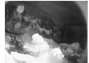
This enzyme/bacteria treated tank rinsed "clean" but left this struvite and sludge behind.
